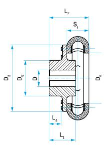
MULTI CROSS FORTE shaft coupling MCF...W
