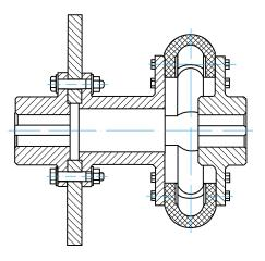
Brake disc coupling MCF...BS
