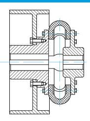
Brake drum coupling MCF...BT
